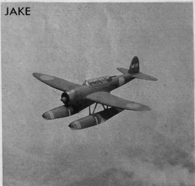
Jake has twin floats, is used mainly for reconnaissance but has attacked Allied shipping with light bombload. Elliptical wing and tail-plane at first confused observers who believed Jake was Val on floats.
